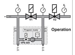
Idle state: Valves 1 and 2 are closed. Pressure build-up: The internal motor pump increases the gas pressure in the test section by approx. 20 mbar compared to the input-side pressure applied to valve V1.
